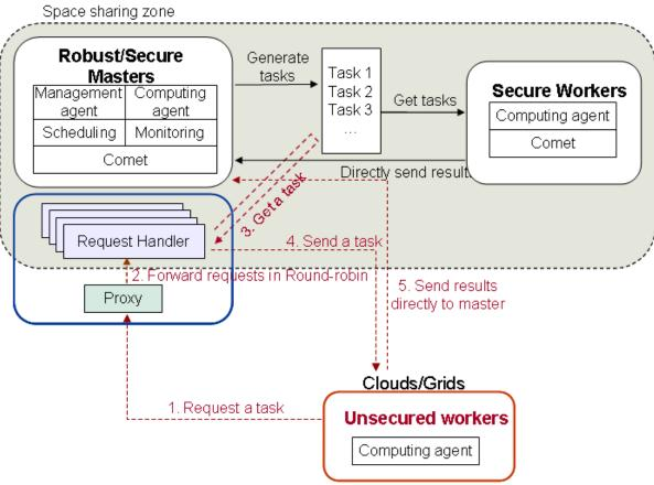
Proxy receives task requests from unsecured workers and forward the requests to one of request handler. Request handler is part of the overlay so as to host Comet space and picks up a task for unsecured workers.
